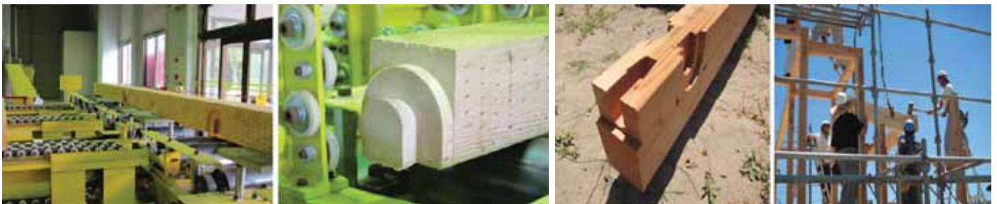
Figure 3: Automation themes in the AEC industry are often associated with the social imaginations of practice. The images above show the automated precut of the timber frame for a custom made beach house which was assembled on site in one day and designed by the firm Bakoko in Japan. The method, which is widely used in Japan, uses robotic machinery that can cut wood joints following Japanese traditional intricate carved joinery and customary assembly methods. (Images courtesy of Alastair Townsend).(Townsend, Alastair. Automation Themes in the AEC Industry Are Often Associated to the Social Imaginations of Practice . Photograph. n.d.)
