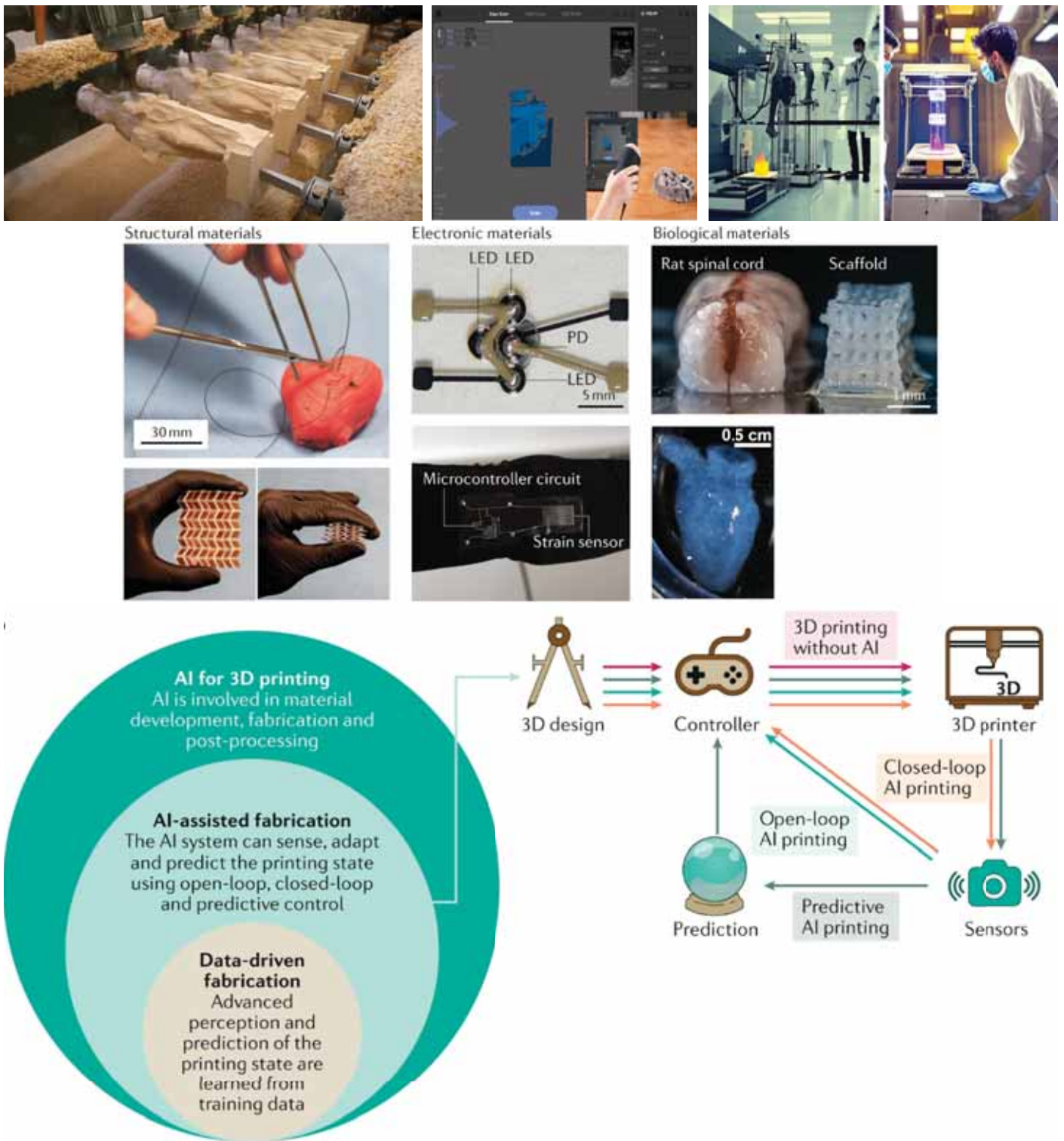
Figure 13: Left top image, A: Production of a wooden carving blank using the copy milling process, Atelier Spiegelhalter, 1990. Middle and left top image: 3D-printed multifunctional materials enabled by artificial-intelligence-assisted fabrication technologies. Image below, B: Overview of 3D-printable functional materials and devices that can be printed with artificial intelligence (AI)-assisted fabrication. Examples of applications for structural materials include a 3D-printed prostate model. (Source: Zhu, Z., Ng, D.W.H., Park, H.S. et al. 3D-printed multifunctional materials enabled by artificial-intelligence-assisted fabrication technologies. Nat Rev Mater 6, 27–47 (2021). https://doi.org/10.1038/s41578-020-002352 )
