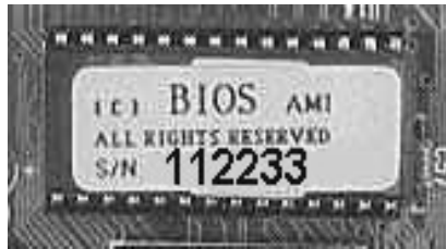
fig.C1.02 – A PC ROM containing the BIOS system
