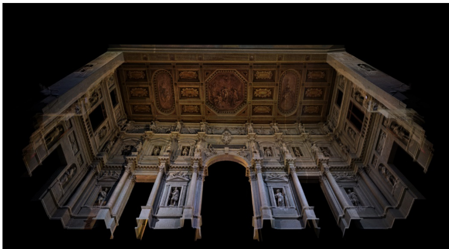
Fig. 4 - Panoramic High Dynamic Range image of the cavea processed from the measurement recordings carried out by a laser scanner
